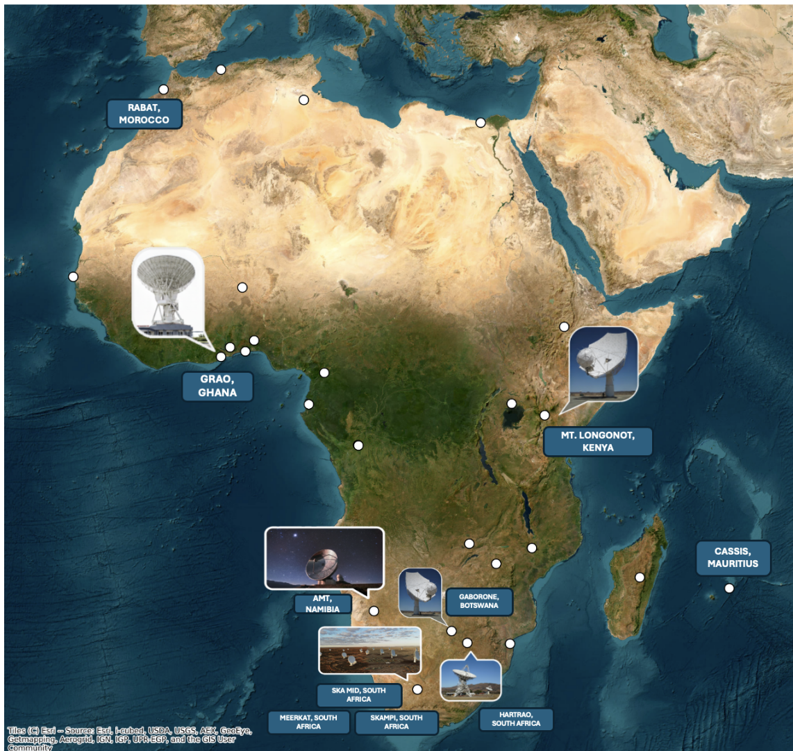
Figure 1: Overview of the locations of the decommissioned satellite antennas previously identified for inclusion in the SKA Partner countries array, together with the potential sites for new SKA-Mid-type antennas across Africa and other planned and current operational antennas. These locations illustrate a possible configuration of a future continental African VLBI array, with maximum baseline length between, e.g. Morocco and Mauritius. The full list of stations is provided in Table 2.
