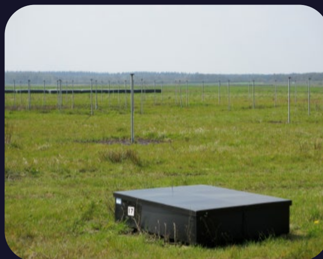
This black box in front of a LOFAR antenna station may not look like much, but it contains a sensitive detector measuring cosmic particles. Credit: Radboud University
