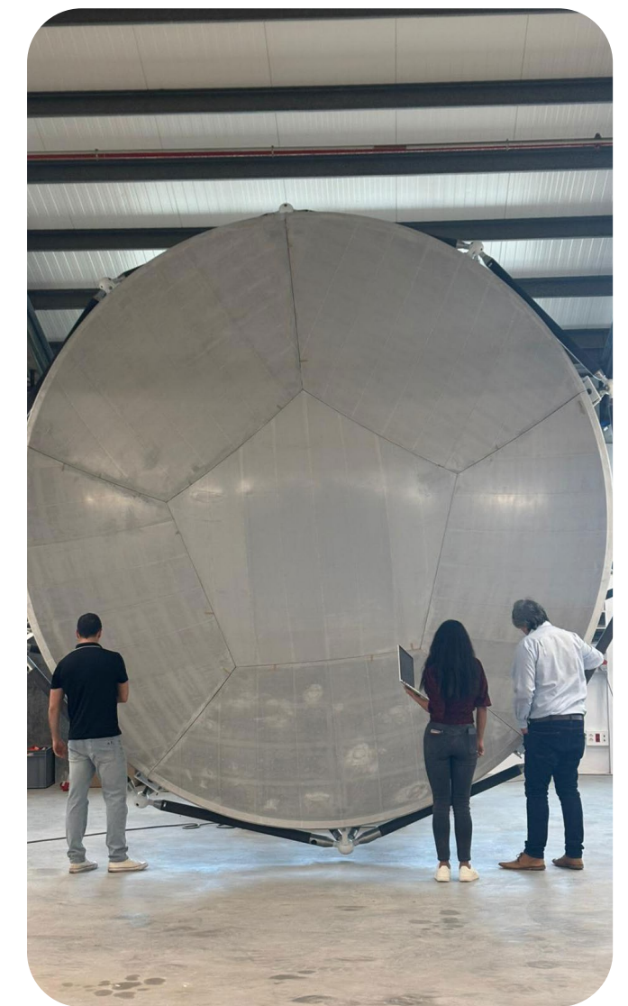
The Spanish-made sub-reflectors measure 4.5m in diameter. Credit: EOSOL and COMPOXI
