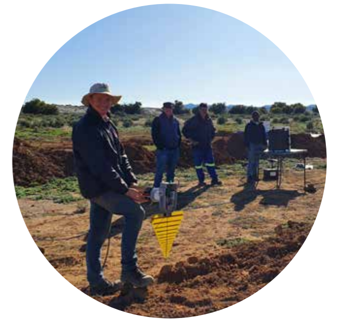
ABOVE: Casey Bryant from MESA Solutions uses an antenna to record emissions from buried cables – part of the team's unique solution to use soil attenuation to absorb Electromagnetic Interference (EMI). Credit: Prof. Reader/MESA Solutions
