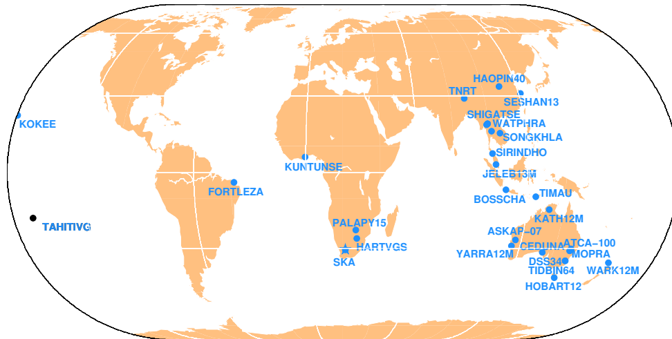
Figure 1: A Southern hemisphere centered network with SKA. At Tahiti site, indicated by a black dot, there is a plan to build a quad-band telescope as one of the geodetic stations while at the other sites radio telescopes are already available (either operating or under signal chain tests).
