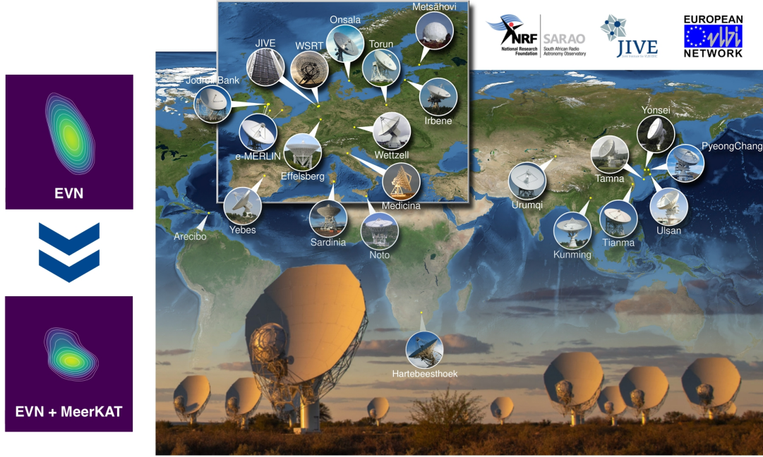
Figure 6: The SKAO precursor MeerKAT observing as a phased-array element of the European VLBI Network. A tied-array beam formed from the MeerKAT dishes is correlated with the other stations of the network, using the same operational model that SKA-Mid will follow. Illustration: Benito Marcote, JIVE. Image credits: MeerKAT image ©SARAO; EVN map image ©Paul Boven, JIVE (satellite image: Blue Marble Next Generation, courtesy of NASA Visible Earth).
